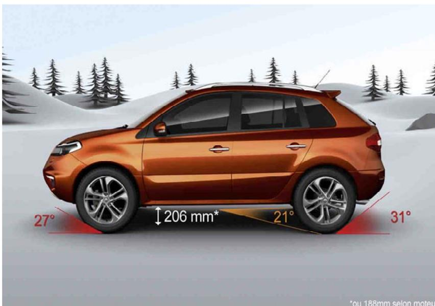
New Koleos boasts real off-road ability and is just as efficient **when used off the beaten track**. Ground clearance of 206 mm (diesel versions: 188 mm) and approach and departure angles of 27 and 31 degrees respectively are
