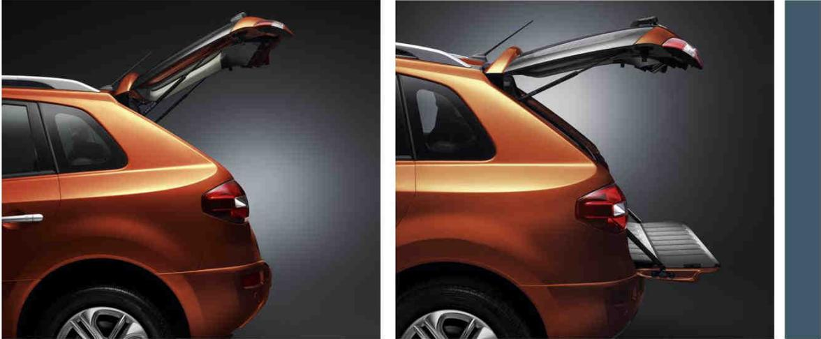
The **'clamshell'-type split-opening tailgate** facilitates access to the boot. The upper part of the hatch permits access to the rear in cramped spaces and allows items of more than one metre wide to be carried. When lowered, the bottom part of the tailgate enables heavy or bulky items to be loaded without getting dirty. It also serves as a robust, handy platform on which items of up to 200kg can be placed.
