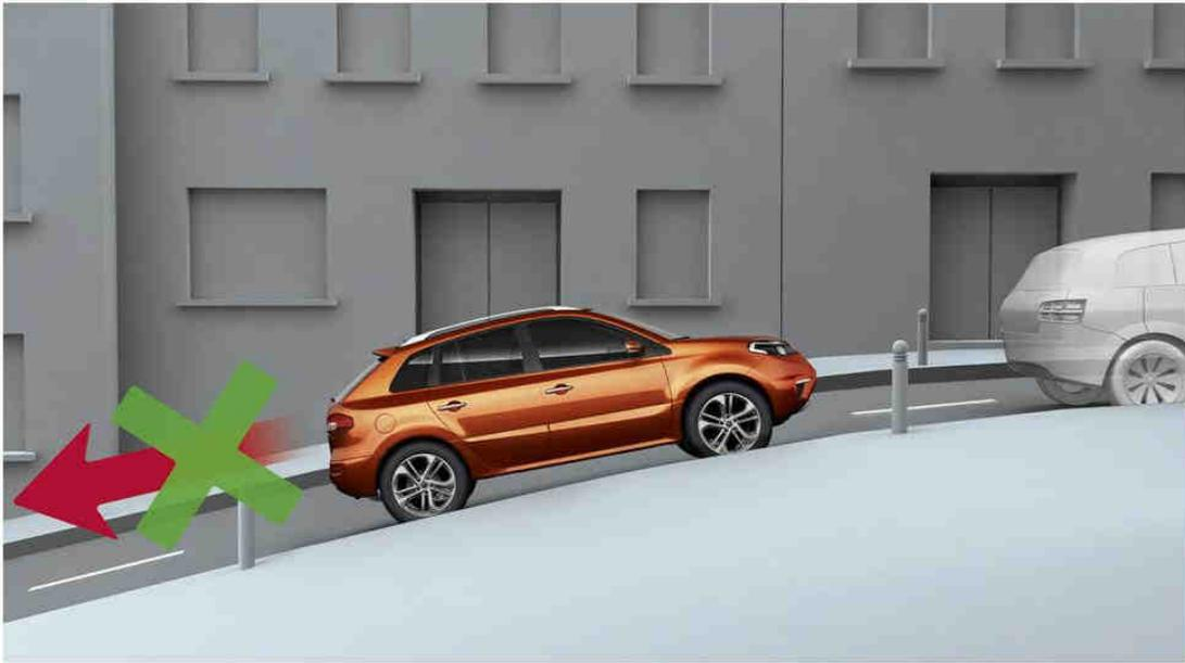
For even safer off-road motoring, Renault Koleos (4x4 version) comes with **Hill Descent Control**. This function is activated via a switch on the centre console and automatically holds the vehicle's speed at a maximum of 7kph on gradients of 10 percent or more.
