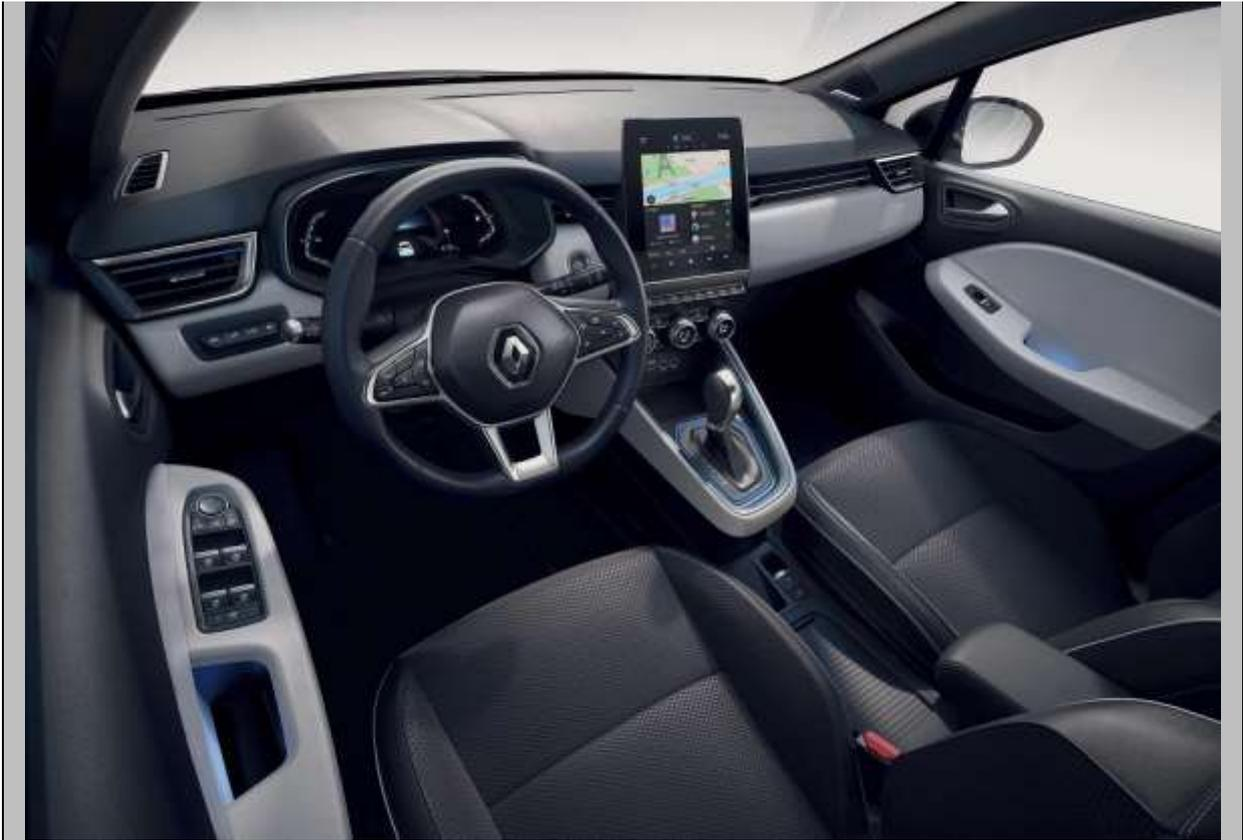
The unique gear stick comes with an 'E-Tech' badge. Lastly, the EV button used to switch to electric mode, provided the battery has sufficient charge, is located below the multimedia screen.
