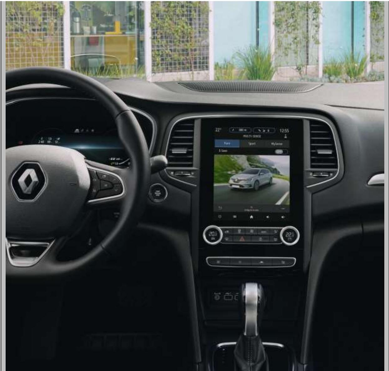
Lastly, the EV button to switch to electric driving (provided the battery has enough charge) is located below the multimedia screen.
